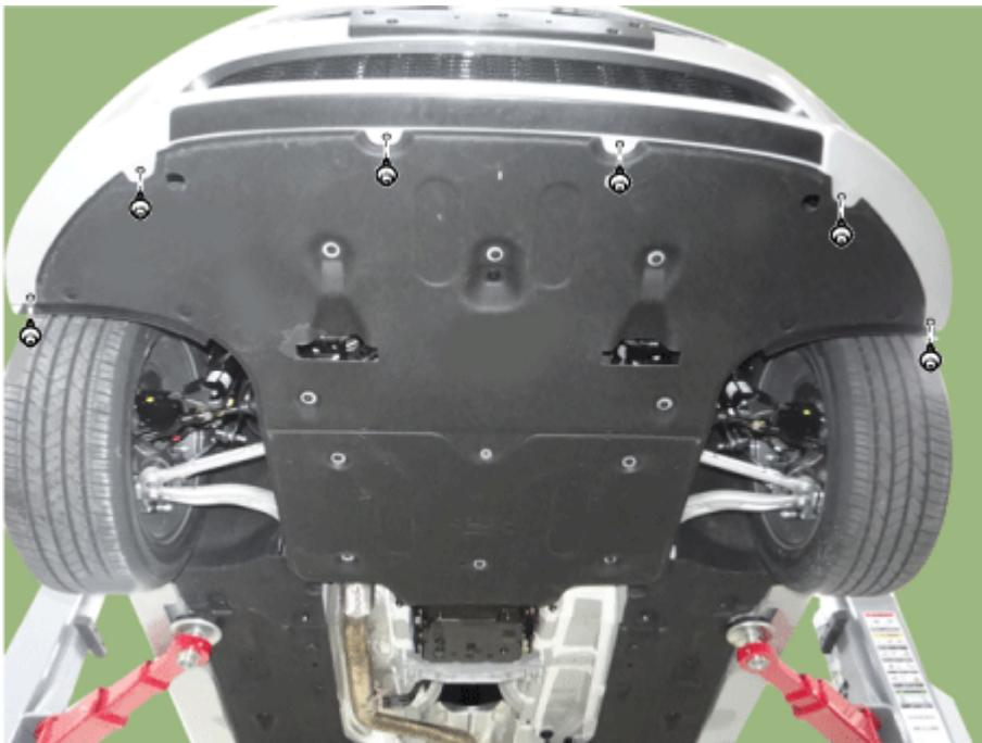
3. Separate the front bumper (A) after loosening the sides mounting clips and screws
