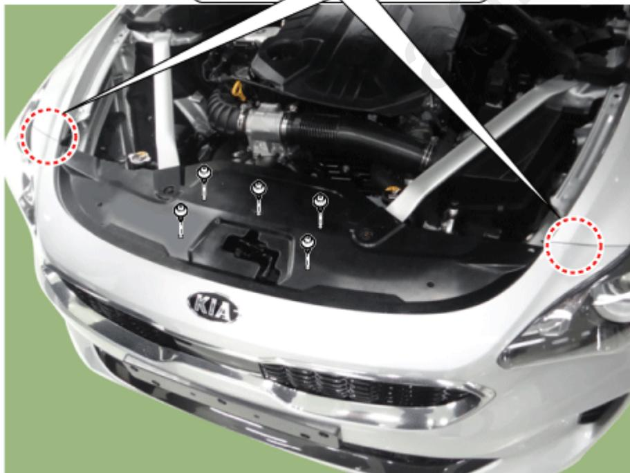
2. Loosen the engine room under cover mounting clips.
